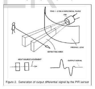
The voltage across the sensors controls a J-FET source follower impedance converter and thus modulates the output current of the PIR detector. The two IR sensors are placed in parallel in the device and
